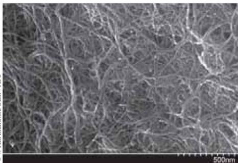
*Carbon nanotubes produced by Prof Veranja Karunaratne at the Sri Lanka Institute of Nanotechnology using Sri Lankan Vein graphite, a type of rock which can contain up to 99% carbon. Plants exposed to carbon nanotubes grow better than usual, making nanotubes a promising ingredient for agricultural fertilizers.*
