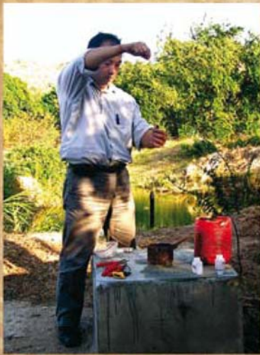
CTD Installation in a monitoring well in Ninh Thuan, Vietnam [Institute of Geological Science, VAST/P.T.K.Nan]
