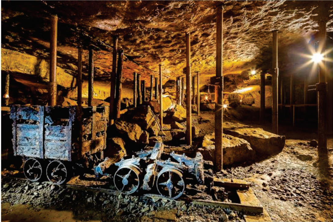
Single wooden pole supports
