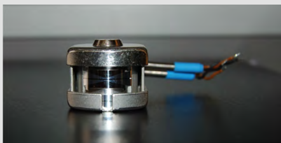
Replay head of a standard magnetic audio tape player ©UNESCO/ Nadja Wallaszkovits
