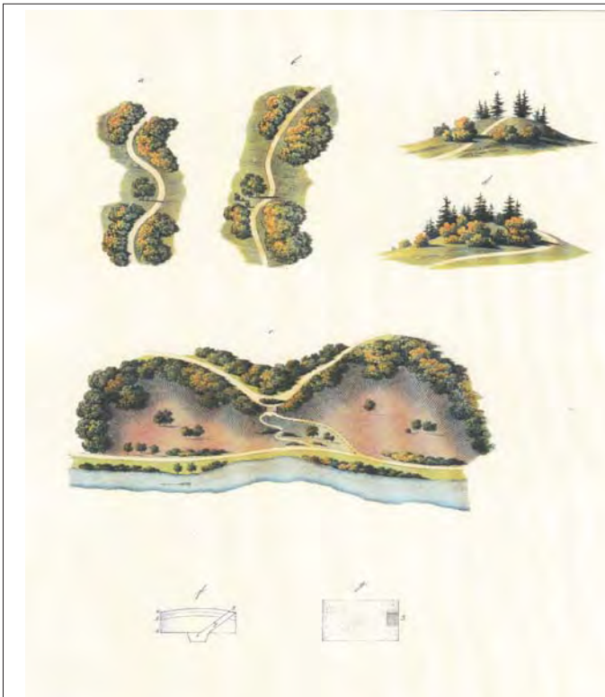
26. a-d Adding motifs to the road turns by putting obstacles e Tracing roads on the slopes (dotted line - wrong) f Cross section and a pavement of a hard-surfaced road
