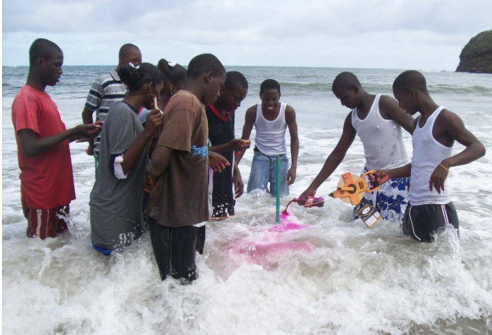
Measuring current direction and speed – La Sagesse Beach, Grenada
