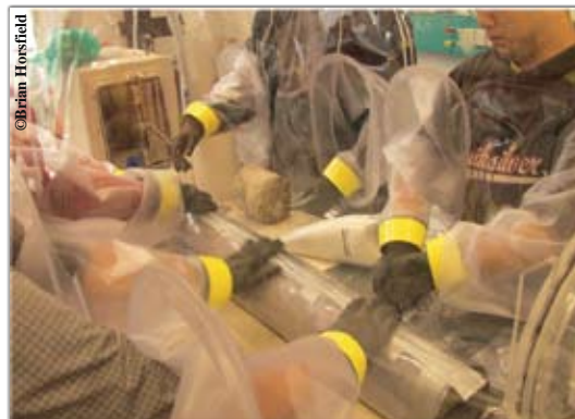
Recovering microbiological life from drill cores demands sterile handling and fluid extraction. Other precautions are necessary when drilling, in order to prevent contamination of a drill hole with microbes from the surface
