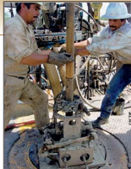
Roughnecks connecting drill pipe joints during the drilling project in the Chicxulub crater on Mexico's Yucatan Peninsula
