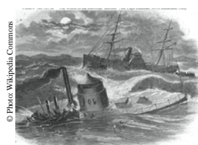
25) The wreck of USS Monitor The United States Ship Monitor pictured in this engraving was the first iron-clad warship. Her low freeboard and heavy turret made her unseaworthy and led to her foundering during a storm in 1862 in the Atlantic Ocean near North Carolina in the USA, with the loss of 16 crewmen.
