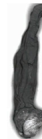
TOP: Wood from the Avondster ship (Galle, Sri Lanka) severely attacked by the shipworm. © MAU
