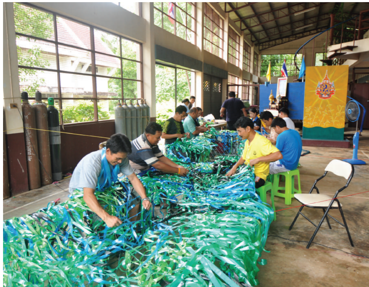
Artificial seagrass can be bought or made by hand. Here, the UAD in Chanthaburi are making their own seagrass by assembling large (approximately 1 metre) fronds on fishing nets. © UAD
