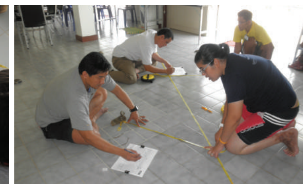
Recording a tie (trilateration using a baseline) during the 'dry' 2-dimensional survey practical session. A measurement is taken from a known point on the artefact to a convenient point on the baseline. A second tie is required to position the point on the artefact. © Christopher J. Underwood
