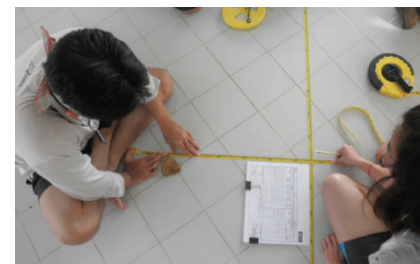
The surveyors are using the survey board to check the 90° offset during the 'dry' practical session. © Christopher J. Underwood
