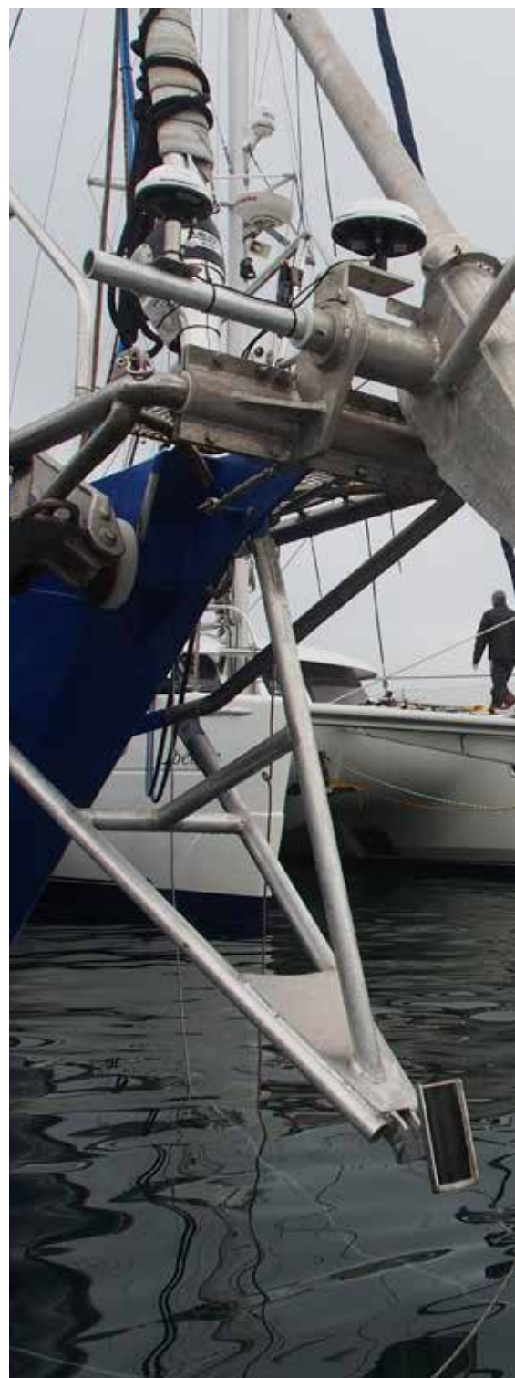
Mounted high-resolution multibeam sonar on the ship Explorer of Sweden during the VEGA 2013 Expedition to Greenland.
