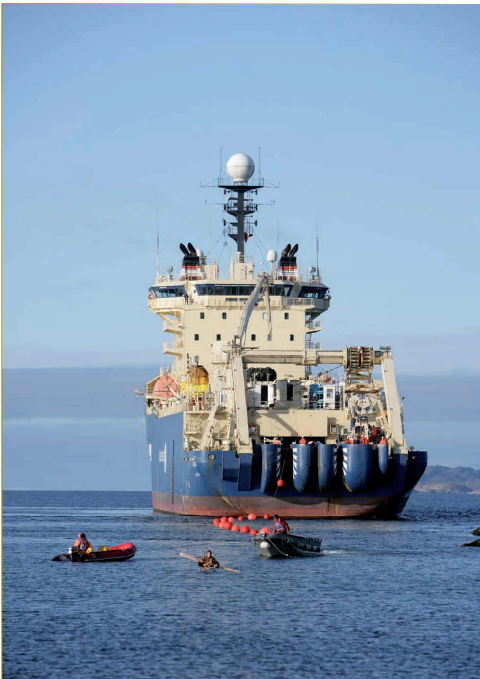
A kayaker hauling ashore the submarine fibre cable at Nuuk, connecting Greenland with Iceland/Europe and Canada/North America. Tele Greenland Ltd.'s cable project is called 'Greenland Connect' (photo: Jørgen Chemnitz/Tele Greenland Ltd.).
