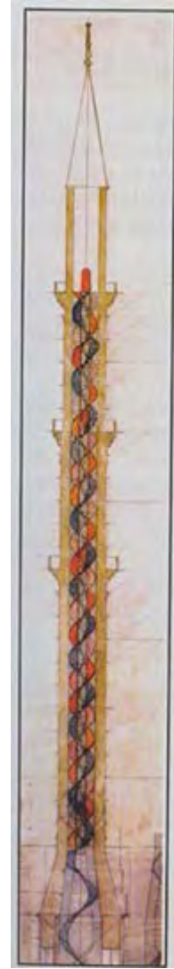
Triple Staircase Details of Selimiye Minarets
