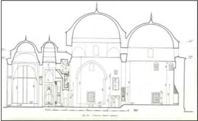
Figure 5: Bursa Yıldırım Mosque Cross Section (Ayverdi)
