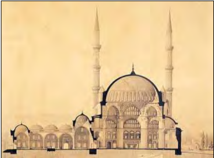
Figure 20: Selimiye Mosque Cross Section (S. Çetintaş)
