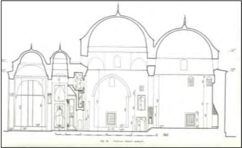
Figure 5: Bursa Yıldırım Mosque Cross Section (Ayverdi)
