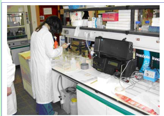
Photo 1. Fluorescence determination with use of spectrofluorometer.
