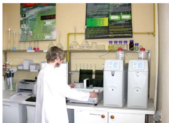
Photo 2. Chromatograph for analyzing ions in water samples (European Regional Centre for Ecohydrology under the auspices of UNESCO, Lodz, Poland; photo: K. Izydorczyk).
