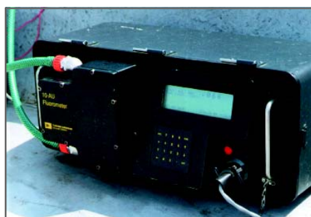
Fig. 7.6 A flow-through fluorometer can be used for monitoring phytoplankton populations in reservoir (photo: M. Lzydorczyk)
