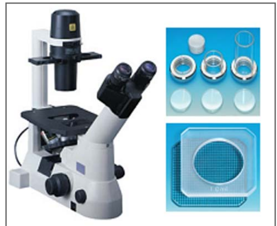
Fig. 7.5 Utermöhl counting technique using a counting chamber and inverted microscope. (photo: Department of Applied Ecology)
