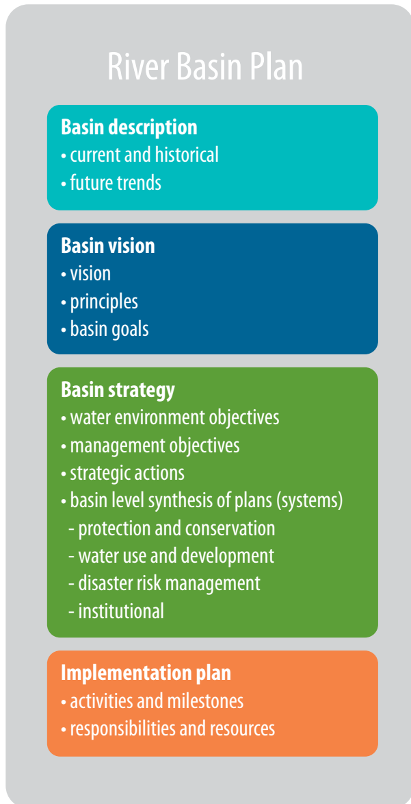
Figure 29: Structure of a river basin plan
