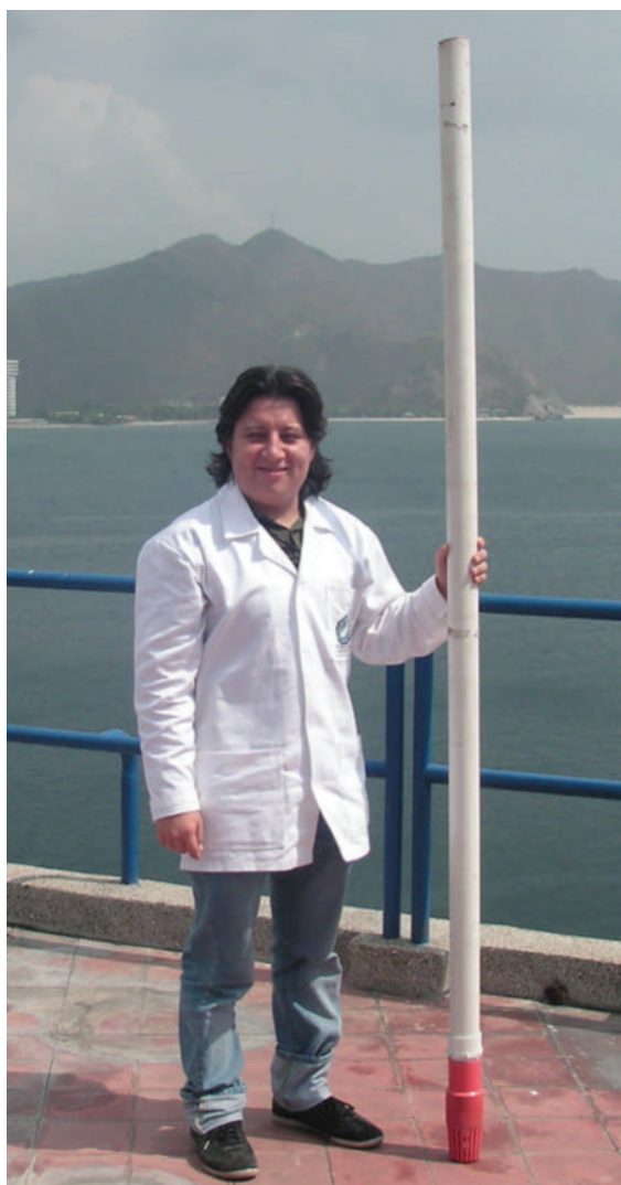
Figure 8. Sampling tube (> 2 m) with a check valve at the bottom end, used by INVEMAR, Colombia.
