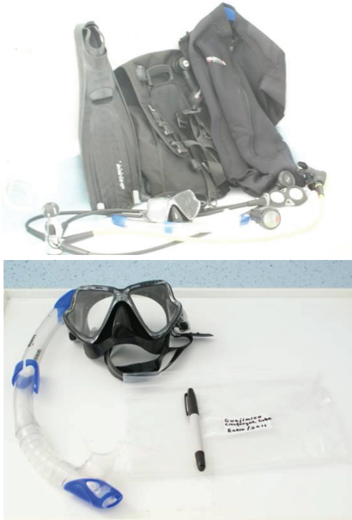
Figure 1. Some of the basic equipment for collecting substrate samples (macroalgae). Top: Scuba equipment; bottom: light snorkelling equipment, plastic bags and indelible marker.
