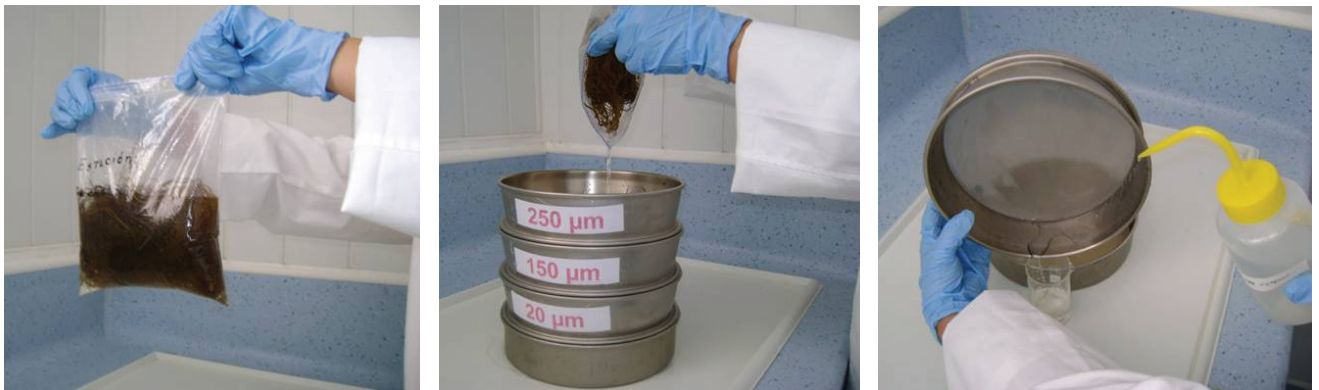
Vigorously shake the bag for two minutes. Filter through three sieves (250 \mu\text{m} , 150 \mu\text{m} and 20 \mu\text{m} ). Rinse and retrieve the residue contained in the 20 \mu\text{m} sieve with filtered seawater.
