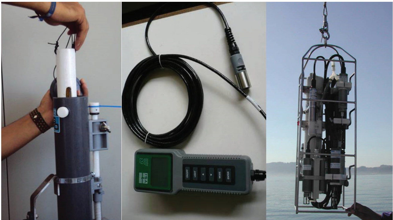
Figure 1. Left: using an immersion thermometer inserted directly into the water-sampling bottle. Centre: YSI multiparameter probe for measuring temperature and salinity. Right: CTD (conductivity, temperature, depth) multiparameter probe attached to the winch of the boat before being cast.
