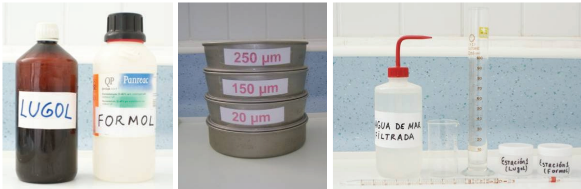
Reagents (Lugol's iodine and formalin) Sieves with different mesh sizes Filtered seawater and some of the equipment (test tube, pipette, plastic vials)
