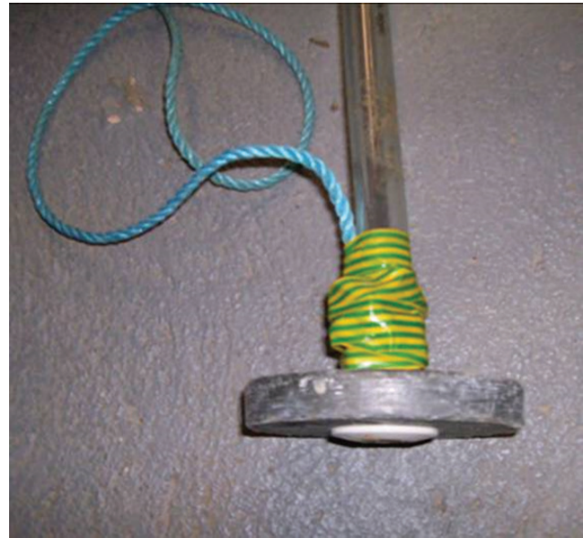
Figure 5. Lund's tube sampler with disk-shaped plumb bob that encircles the bottom end of the tube.
