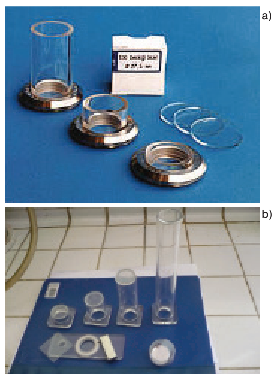
Figure 4. a) Simple sedimentation chambers of 25, 10 and 5 ml; b) Combined sedimentation chambers: bottom sedimentation plate with cover slide and key to unscrew the metallic ring (front) and sedimentation cylinders of 10, 25, 50 and 100 ml (rear)
