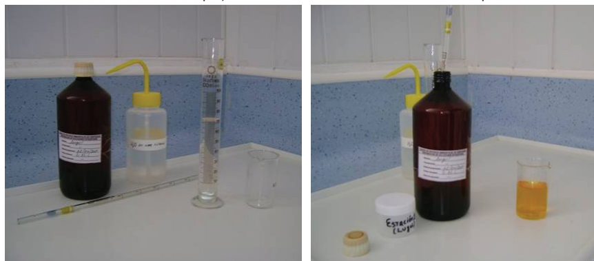
Measure the final volume of the sample. Add the neutral solution of Lugol's iodine to preserve the sample.
