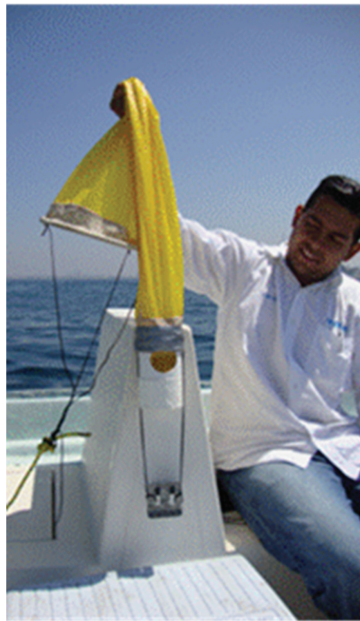
Figure 3. Left: plankton net with a cod end with a stopcock for unloading the sample. Right: plankton net with a cod end, or collection cup, and a weight attached for the descent into the water (model provided to participants in Project RLA/7/014).
