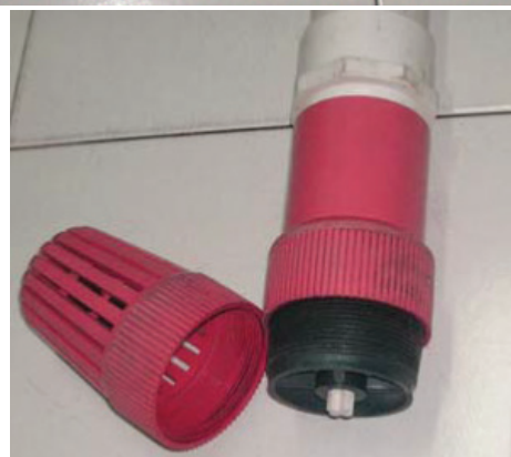
Figure 9. Close-up of a check valve used with a tube measuring two inches in diameter (Photo: INVEMAR, Colombia).
