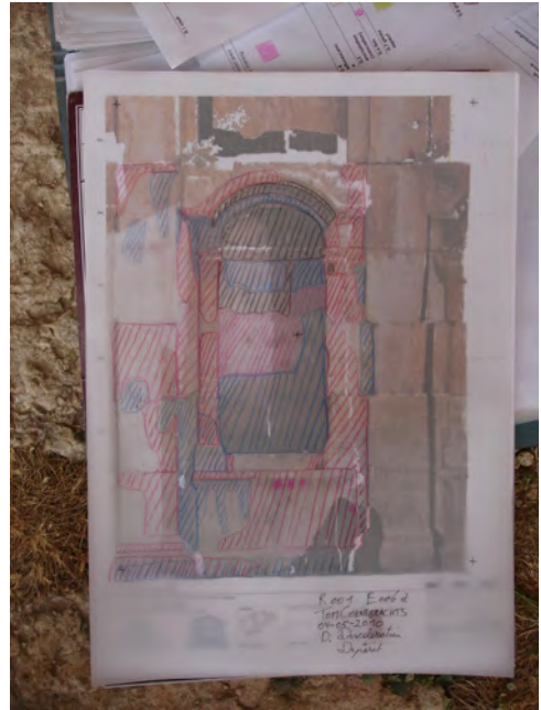
Figure 8.1: Graphical survey of the surface degradations on transparent sheets with coloured pencils.
