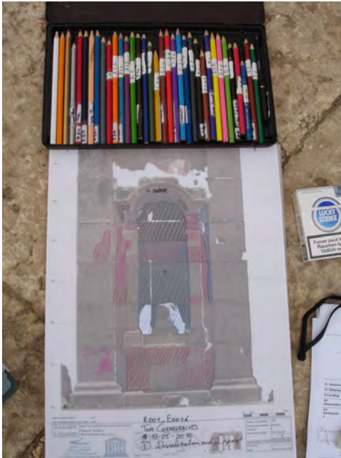
Figure 8.1: Graphical survey of the surface degradations on transparent sheets with coloured pencils.
