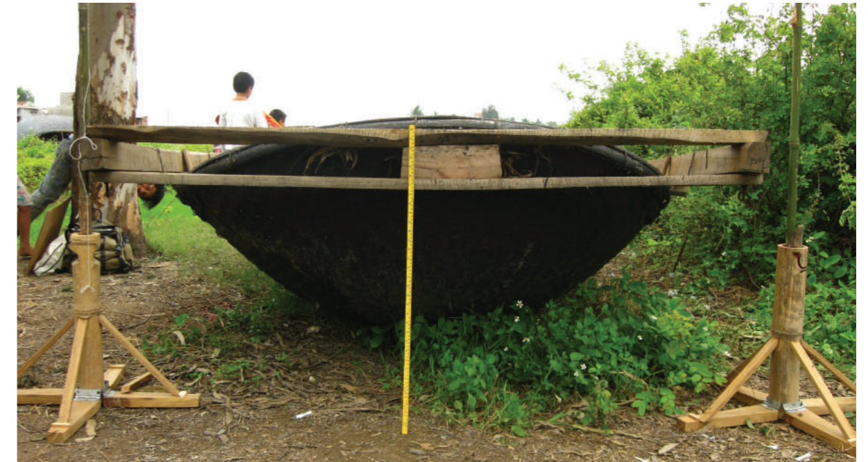
Boat Tuong 14 with stands along which measure tapes and references can be strongly fixed. Mr. Toan Huyen's boat yard, Huong Hoc village, Quang Ninh province. © Charlotte Minh-Hà Pham
