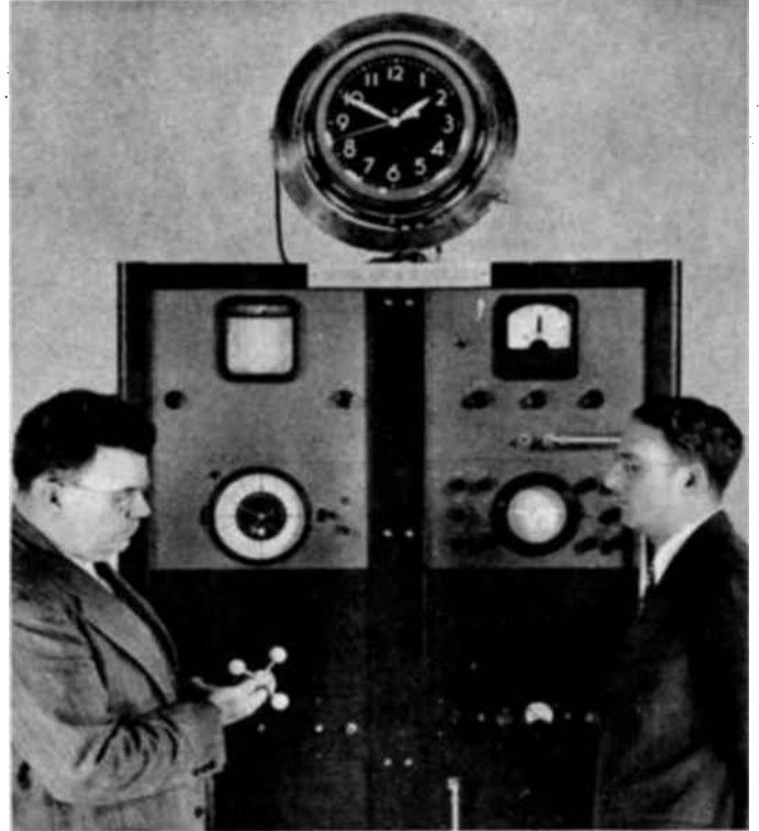
A CLOCK FOR THE ATOMIC AGE. In a radical departure from all conventional methods of measuring time, an atomic clock—invariant with age and for the first time independent of astronomical observations—has been developed by the National Bureau of Standards in Washington. Based on a constant, natural vibration frequency of atoms in the ammonia molecule, the atomic clock is a scientific achievement which offers an entirely new primary standard of frequency and time. Its principle promises to free man from age-old methods of fixing time by the daily rotation of the earth on its axis, as it revolves around the sun. The primary standard, the earth, is very gradually slowing down and, in addition, unaccountable fluctuations in the rate of rotation have sporadically lengthened and shortened the day. The new method offers an invariant master clock against which the variation in timekeeping of the earth could be measured. This photo shows Dr. E. U. Condon, Director of the National Bureau of Standards, (left) and Dr. Harold Lyons, inventor of the clock, in front of the panels which control it. Dr. Condon is holding a model of the ammonia molecule whose absorption of radio energy provides the invariant frequency upon which the principle of the clock is based.
