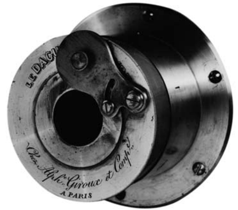
Plate 132 Shutter and lens of an early French daguerreotype camera (c. 1840). © Austrian Archives/Corbis/Cover
