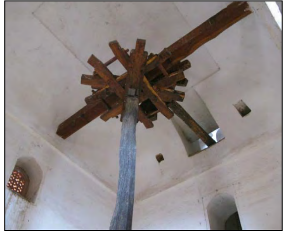
The Persian wheel system for the final stage of lift reinstalled in 2006-2007
