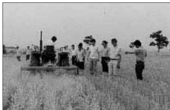
Photo 5.7: Subsoiler in operation on large farmfields
