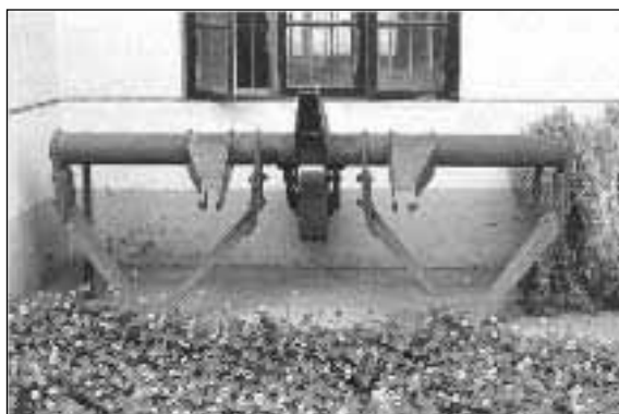
Photo 5.6: (Double) V-shaped subsoiler
