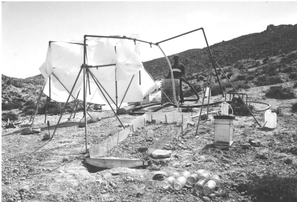
Figure 5.2 Mobile rainfall simulator (left) and Kamphorst infiltrometer (right) used in the Amrich jessr experiments
