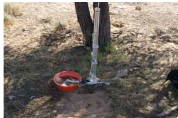
Figure 5 and 6. Soil sampling (above) and infiltration test (below) © Ken De Sadeleer, University of Gent
