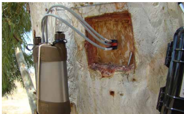
Figure 6. Sap flow meter installed in a Eucalyptus camaldulensis trunk © Mojtaba Pakparvar
