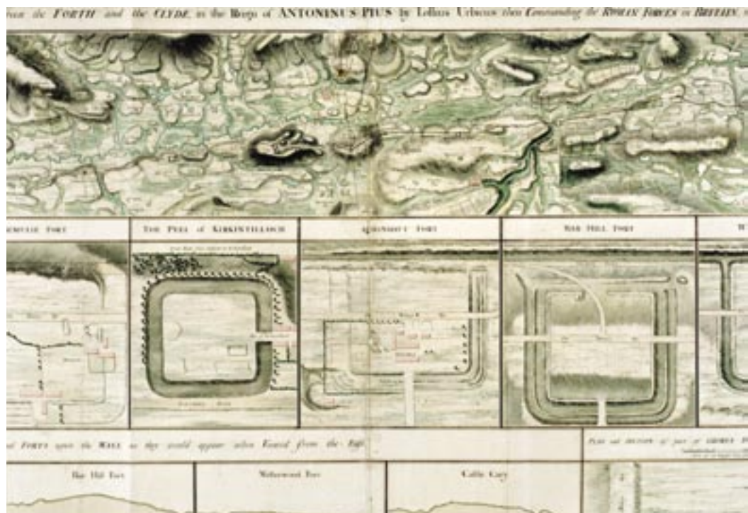
William Roy surveyed the Antonine Wall in 1755. His map of the Wall was accompanied by plans of the forts and sections across the frontier. This section illustrates the central sector.
