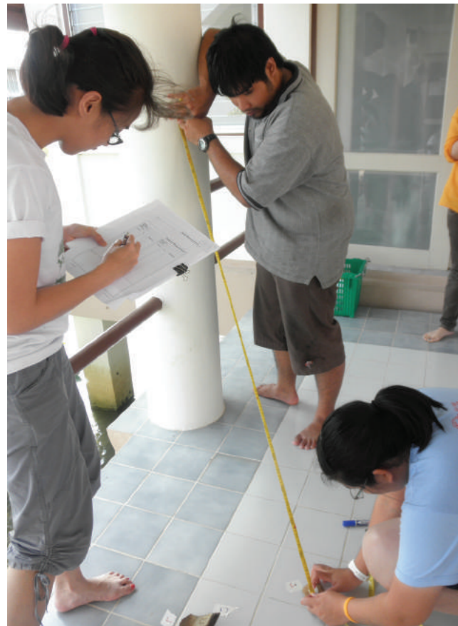
LEFT: Taking a direct survey measurement from a control point to a detail point on an artefact. © Christopher J. Underwood
