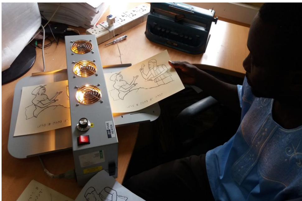
A Brillist passing the photocopy diagram on the zychem paper through the zy fuse heater for the diagram to be felt by the visually impaired
