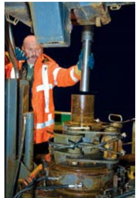
FIGURE 4 The cores were taken with an installation placed at the stern of the research vessel.
