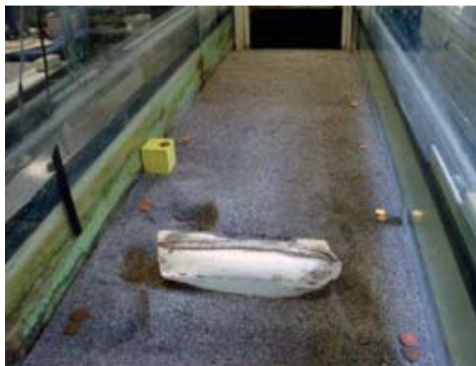
FIGURE 1a-b Bi-directional pump system and the placement of the model vessel on the mobile bed. The coins and blocks represent reference points to enable stitching of laser scans so larger surface areas can be recorded.
