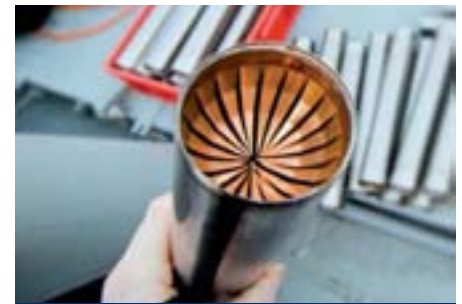
FIGURE 3 The Ackermann tubes are 350mm long and 66 mm in diameter. The samples are undisturbed and completely sealed off to prevent light coming in. Photo: P. Voortuis/Highzone Photography.
