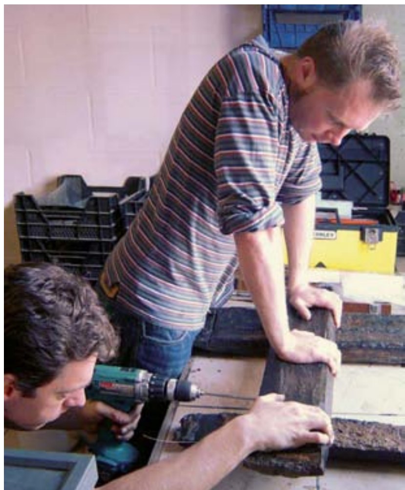
FIGURE 5 Dendrochronological analysis of wood from a barrel provided a terminus post quem of 1735 for the sinking of the ship. © VIOE
