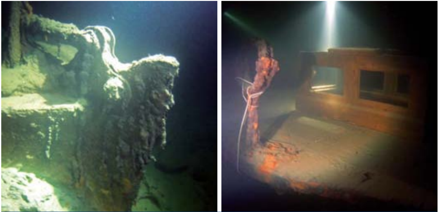
FIGURE 3a-b The intact sternpost of the 90-metre wreck of SS Ingrid Horn is almost covered in sediment. We can also see that the wooden structures are almost entirely intact. Photo: Jakob Selbing
