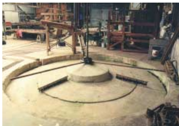
King Edward Mine (A5, tin dressing plant Listed Grade II*). A convex buddle, used to concentrate fine-grained tin-ore.
