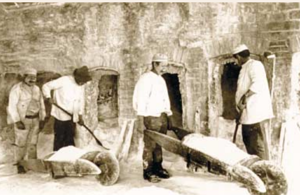
Collecting white arsenic from the flues, Roseworthy arsenic works (that served mines in A3i and A5).
