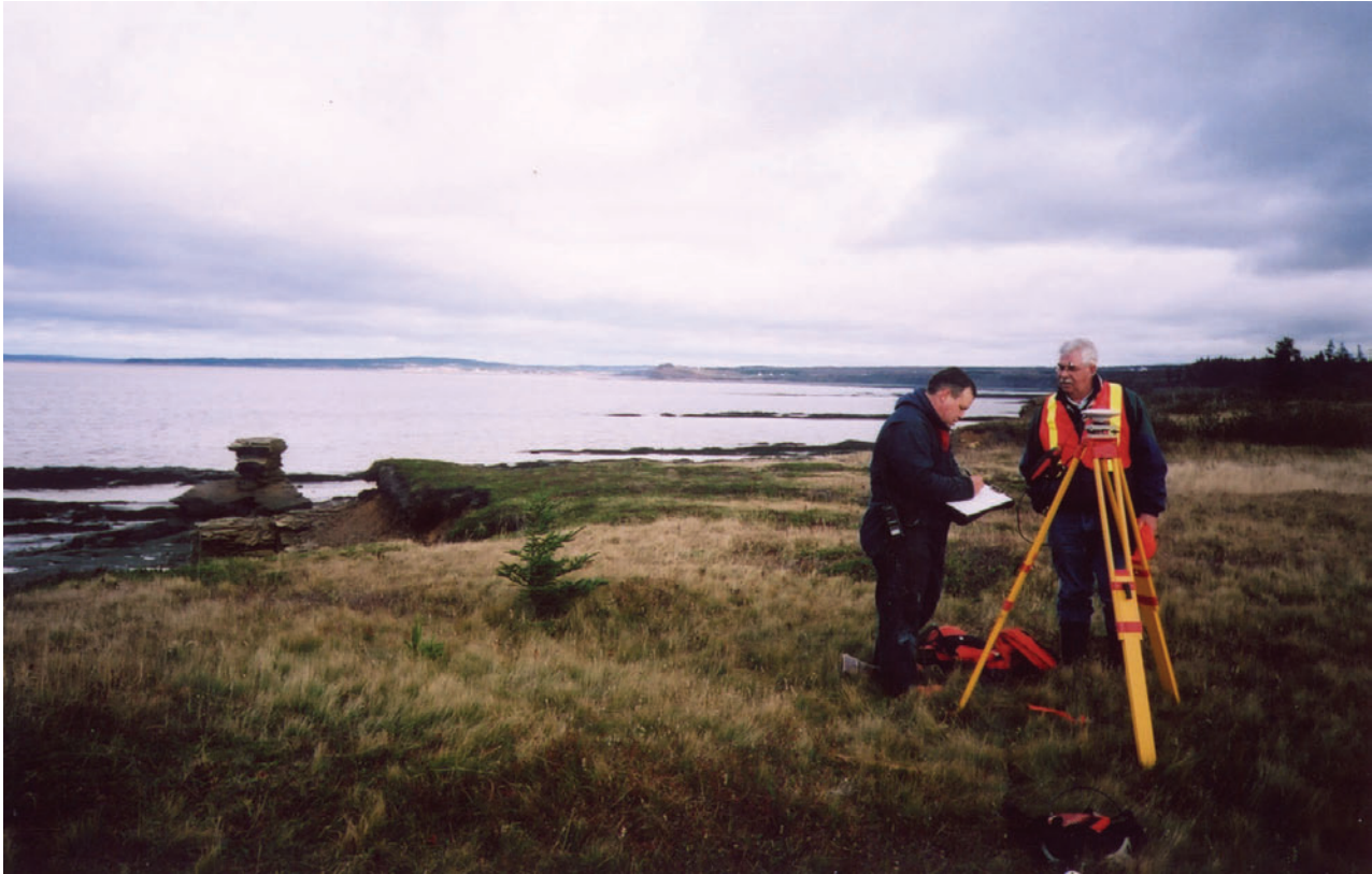
Figure 2. DNR surveyor Jeff Hingley, with Sandy Cameron, establish a benchmark near Ragged Reef Point (see Fig. 1 for location).
