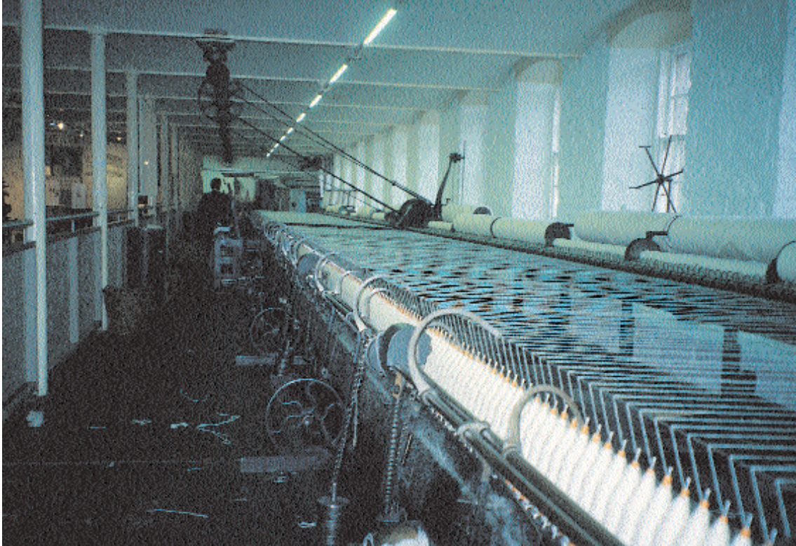
Mill Number Three, New Lanark, with Platt Brothers mule of 1891 under a brick arched, iron-framed ceiling.
