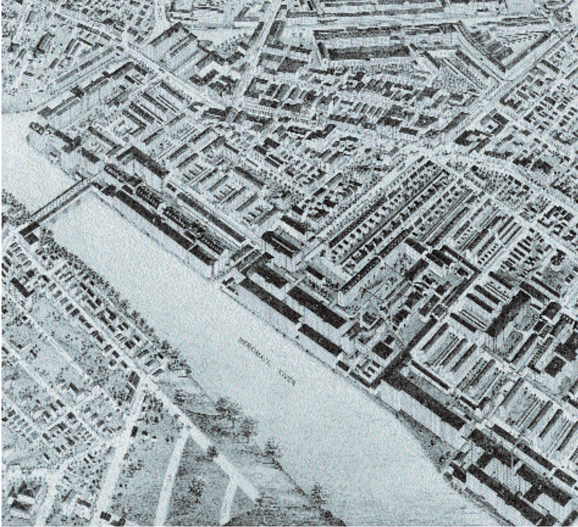
Bird's Eye View of Lowell, Mass., USA, in 1876. Cotton mills (2 Merrimack, 3 Laurence, 6 Boott, 7 Massachusetts, 9 Tremont and Suffolk) are each aligned axial to or parallel to their power canals, with rows of mill girl boarding houses perpendicular to them. Massachusetts Mills are a mirror image to the layout of New Lanark. (American Textile History Museum, Lowell, Mass.)
