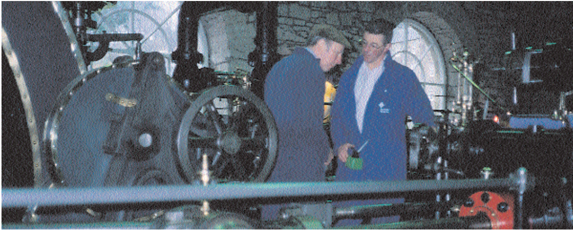
250 hp twin tandem compound engine by J. Petrie of Rochdale, built 1912
