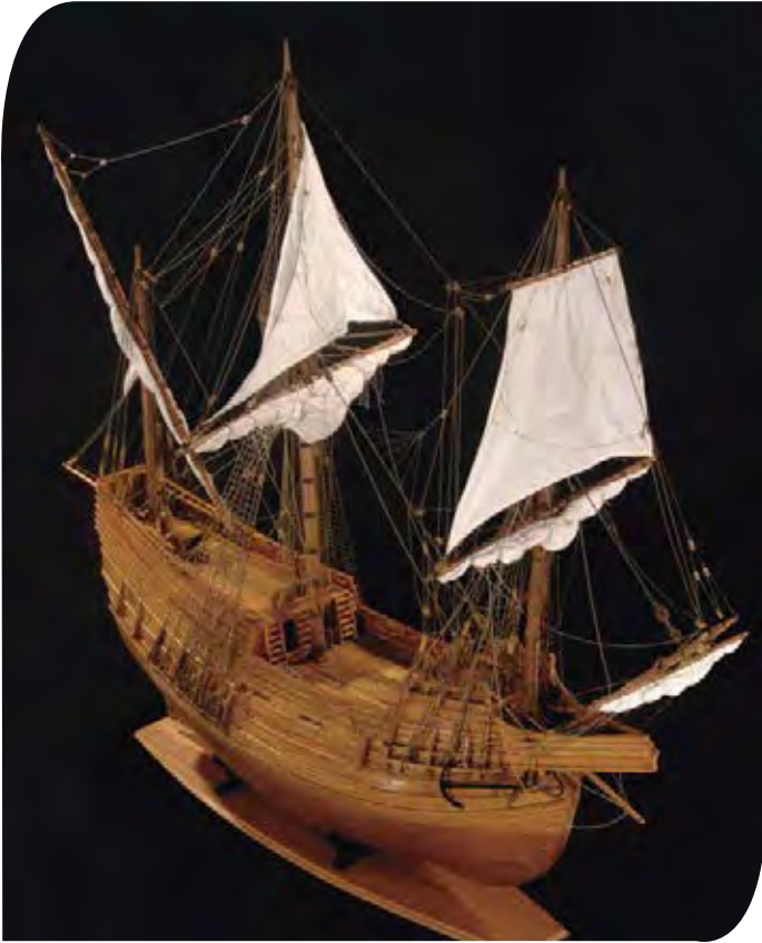
Figure 3.19 1:20 scale model of the 24M vessel based on archaeological evidence recovered from Red Bay. Parks Canada/G. Vandervlugt
