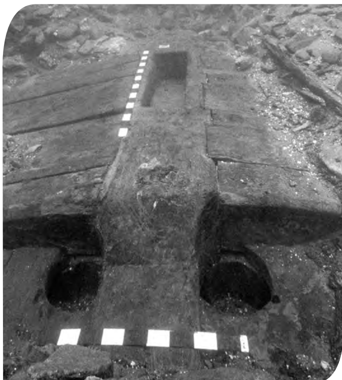
Figure 2.18 Mast step of the 29M vessel. Parks Canada/D. Pagé
