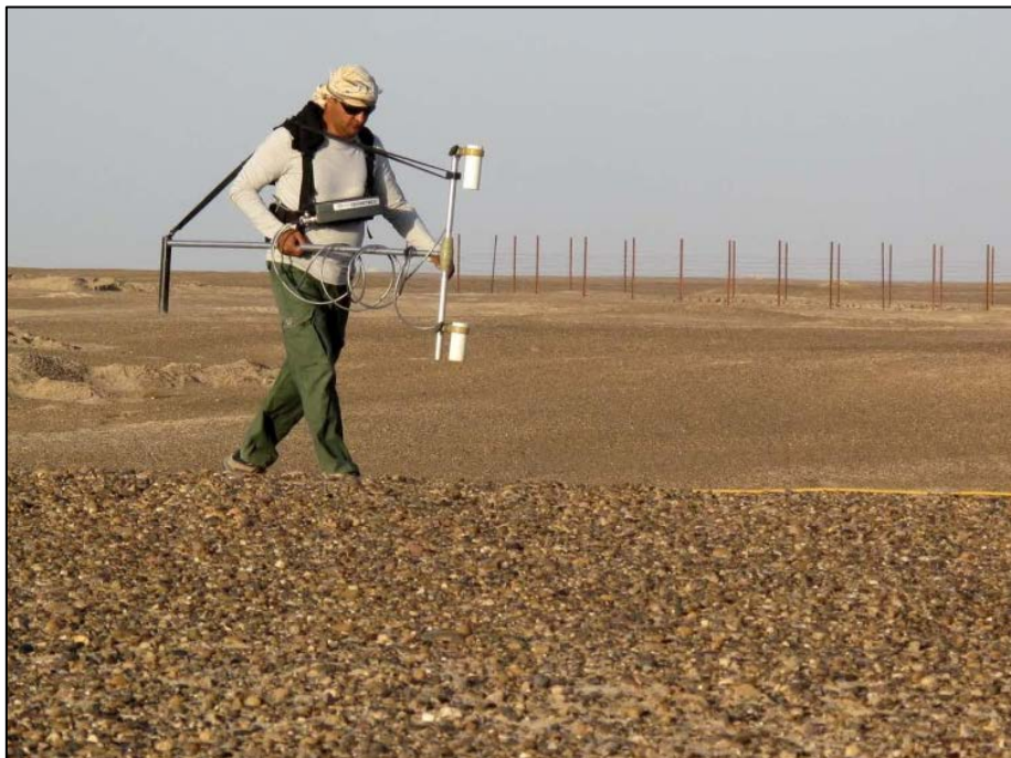
Photo 13. Method of magnetometric scan in the potential northern cemetery of Shahr-i Sokhta
