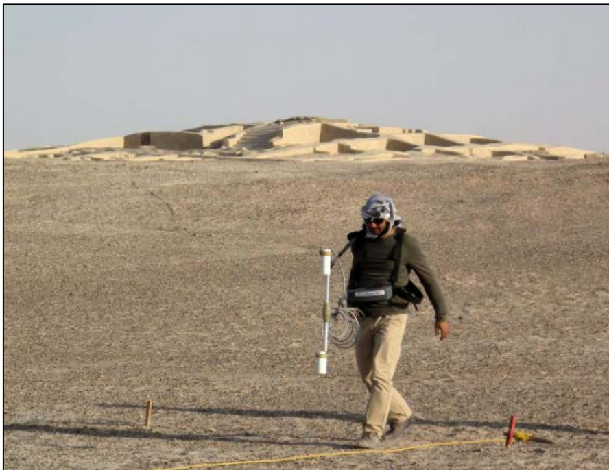
Photo 15. Method of magnetometric scan south west of the monumental building of Shahr-i Sokhta
