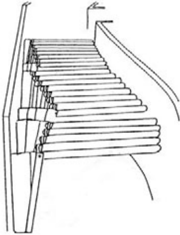
18. Sketch of Utzon's corridors based on mock-up model.
