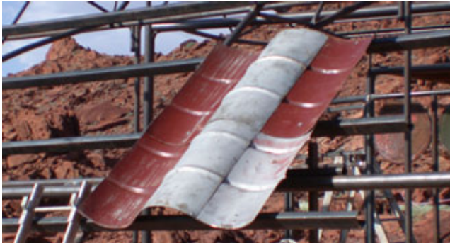
Fig. 8: Roofing tiles from recycled oil drums.
