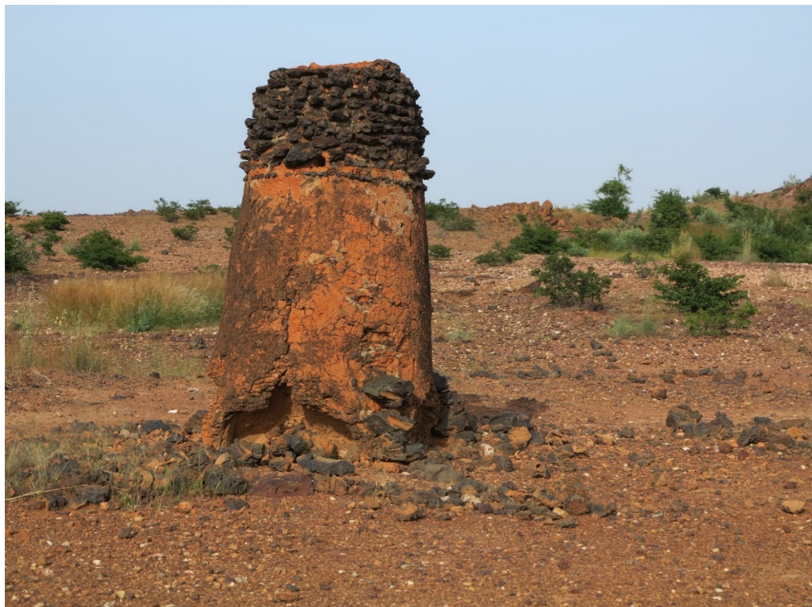
Furnace, natural air draft type, Tiwêga
