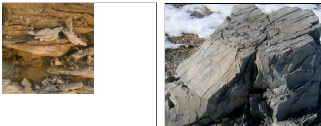
Fig.4-61.A sample of lamination and shattering of lime stones and black stones (Parse-Pasargadae Research Foundation Archives)
