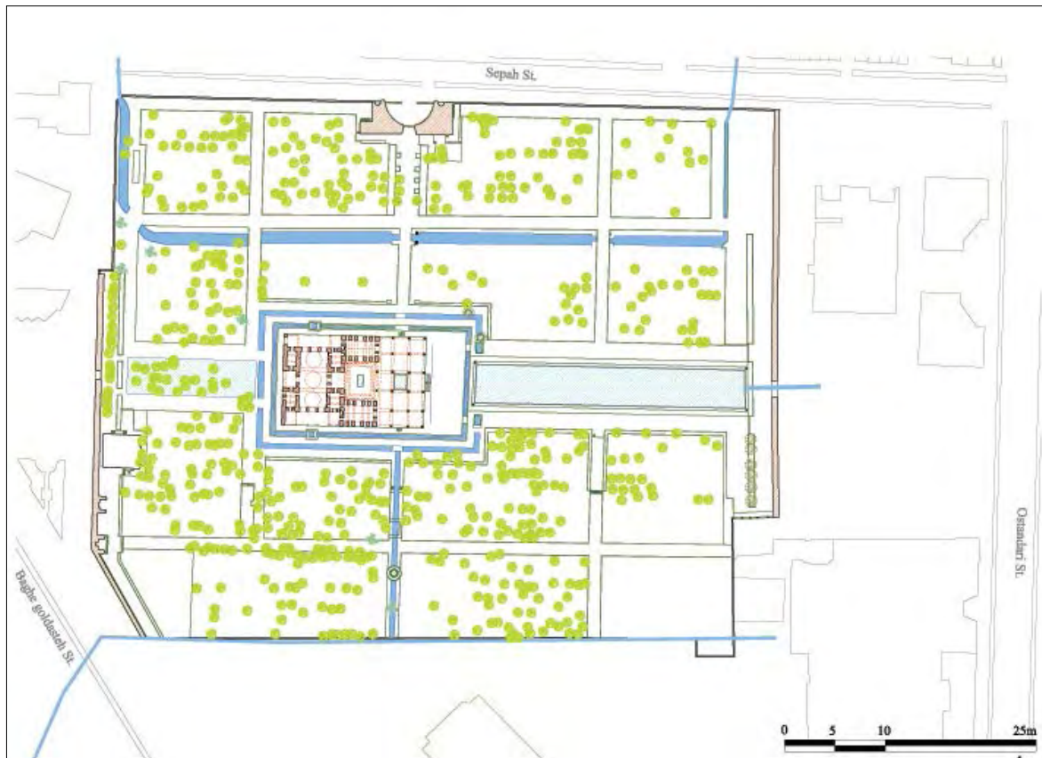
Fig .2-96. The course of circulation of water in Bagh-e Chehel Sotun and surrounding (NHBI, Base)
