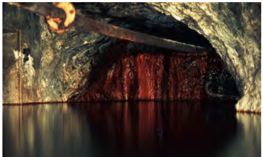
002 114 THE SHUTDOWN PROCEDURES INCLUDE THE GRADUAL FLOODING OF THE XI th LEVEL.
