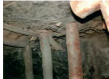
002 074 THE IDRIJA DRIFT SUBLEVEL MINING METHOD BY USING A REINFORCED BACKFILL – CONCRETE
