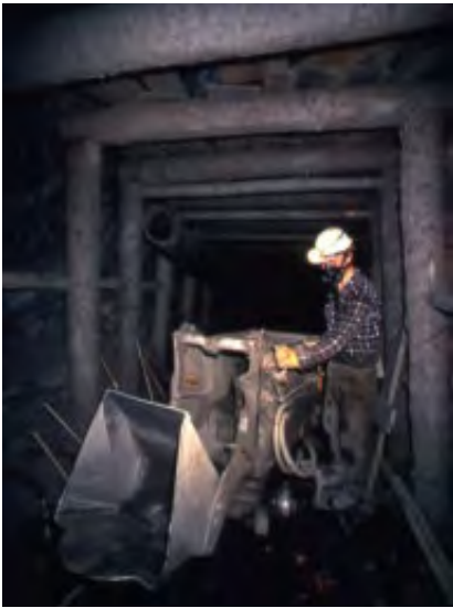
002 072 EIMCO PNEUMATIC SHOVEL ON COMPRESSED AIR
