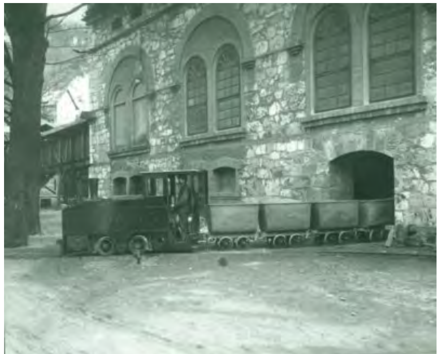
002 146 DEUTZ MANNHEIM PETROL LOCOMOTIVE FOR TRANSPORT OF SMELTING REMAINS, EARLY 20 TH CENTURY
