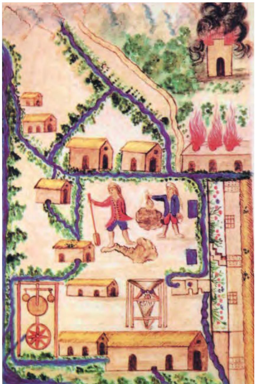
001 061 ETCHING OF THE AMALGAMATION OF SILVER WITH MERCURY. (MARTÍNEZ COMPAÑON COLLECTION. LIBRARY OF THE ROYAL PALACE IN MADRID)
