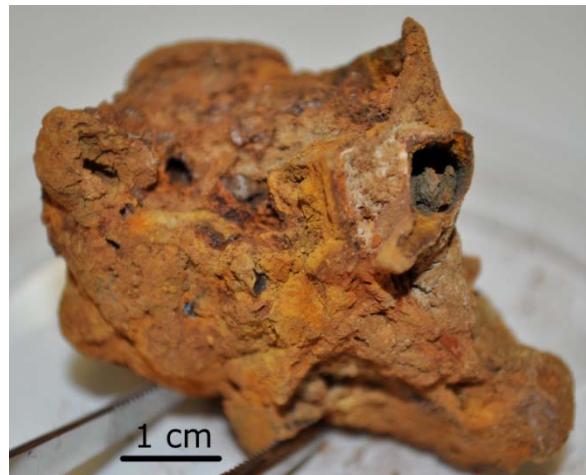
Figure 4. A foot shaped sample of rusticle taken from the RMS Titanic in 1991. The chemical reactions of iron oxide produce the autumnal colours of red, orange, yellow and brown. The large blackish opening on the upper right side of the sample is a channel that circulates water through the rusticle structure.
