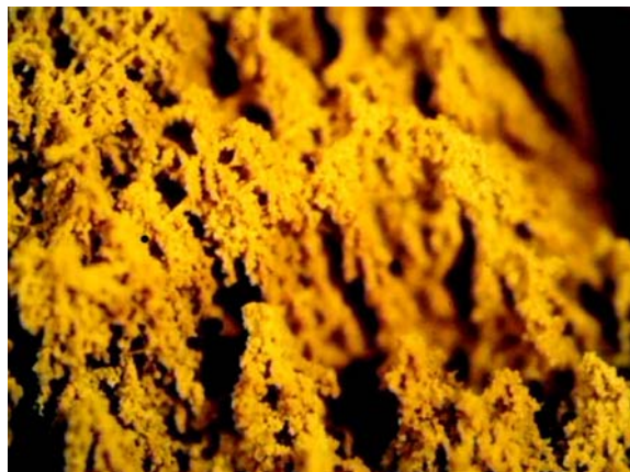
Figure 6. Goethite is an iron bearing oxide mineral occurring inside the rusticle structure.
