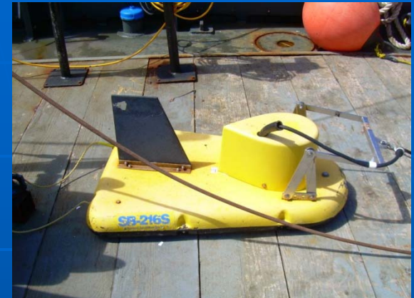
Edgetech SB-216S Subbottom Profiler 2-16 kHz (Chirp)
