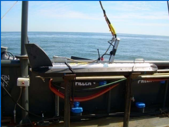
Edgetech FS-2400 Sidescan Sonar 120-410 kHz (Chirp)
