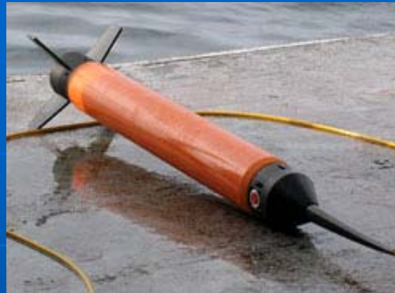
Marine Magnetics SeaSpy Magnetometer 2 Hz sampling rate
