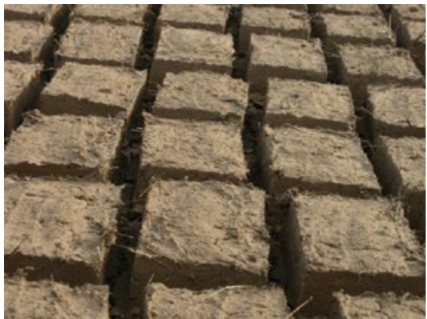
Development of reinforced clay using hay
