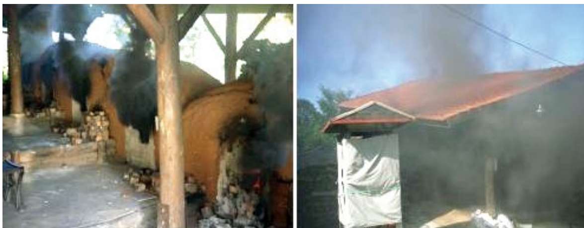
Soot occurring from firing a traditional firewood kiln
