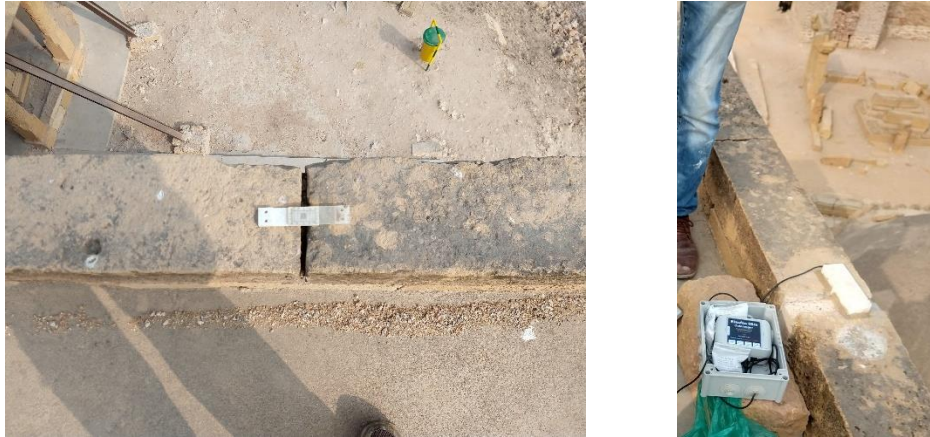
Figs. Jam-1 and Jam-2. JamNizamuddin. A passive crack monitor installed on the roof (l.). A digital crack monitor and datalogger on the roof (r.). ©J.Bell2019
