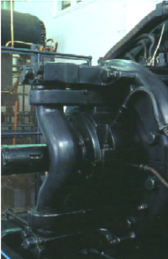
The Alexanderson transmitter, main rotor bearing of alternator, 2001
