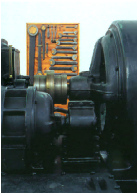
The Alexanderson transmitter, main motor and auxiliary oil pump motor, 2001
