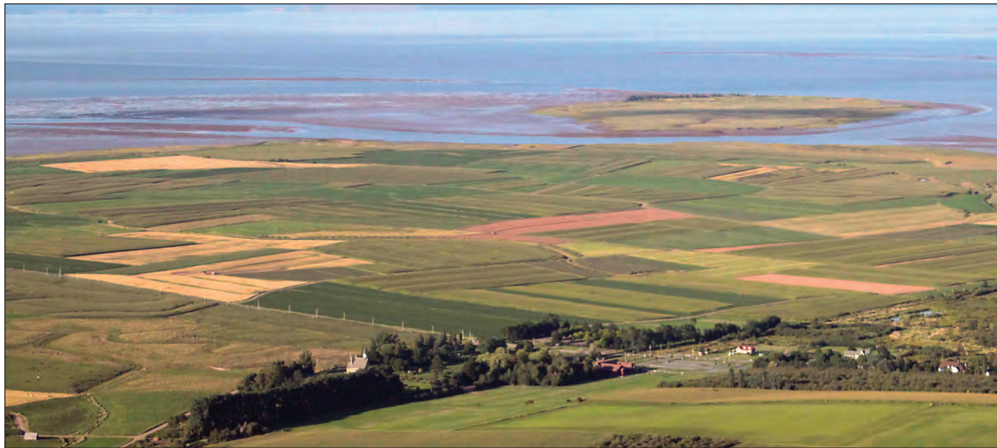
2-7 Fields on the dykelands are shaped to create optimal drainage conditions.
