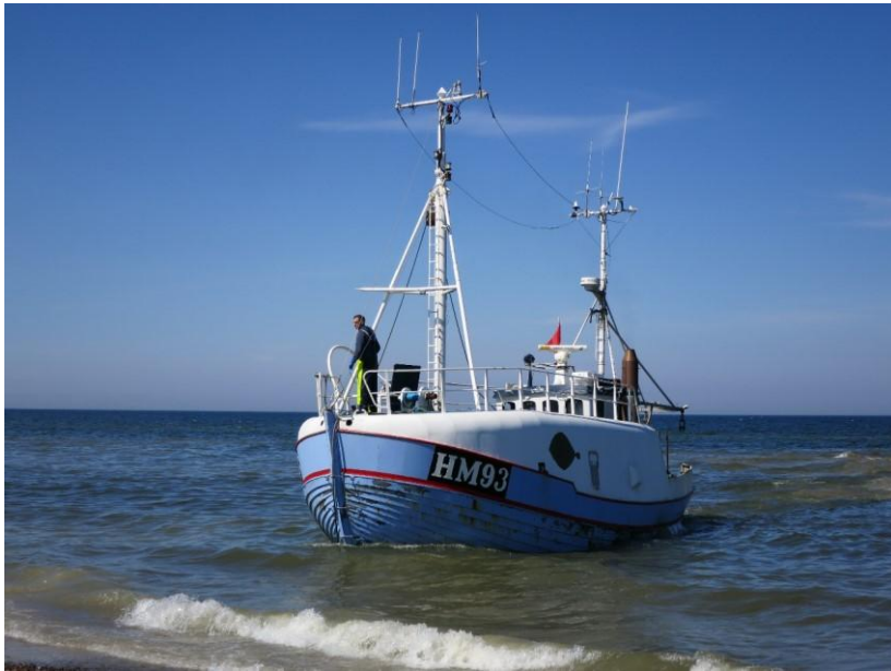
The clinker-built coaster Liv lands at Thorup Strand after a day fishing with Danish seine. May 2016. Photographer: Kirsten Monrad Hansen, Han Herred Havbåd
