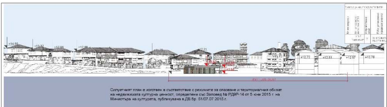
Detail showing how new port-side facilities will be limited in height so as not to impact visually on the buildings of the historic town above. (© Image provided by the State Party)
