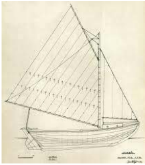
Gaff rigging. Mast, boom, gaff. The triangular sail ahead of the foremast is called a jib.
