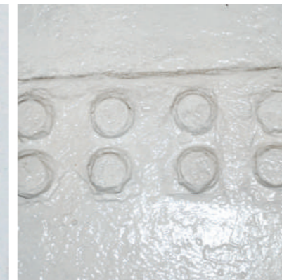
Watertight bulkhead (across the beam of the vessel). © Christopher J. Underwood
