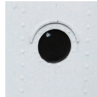
ABOVE LEFT: Riveted hull construction. © Christopher J. Underwood
