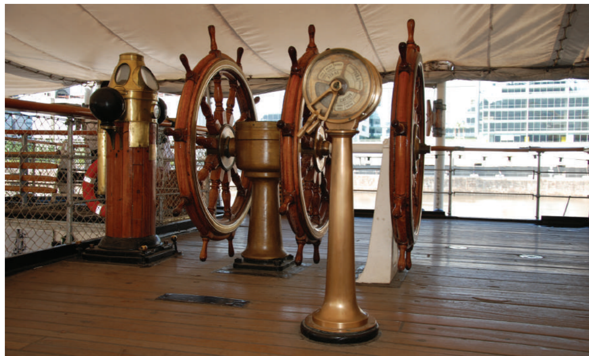
From left to right, ship's navigation compass, ship's wheel and telegraph. © Christopher J. Underwood
