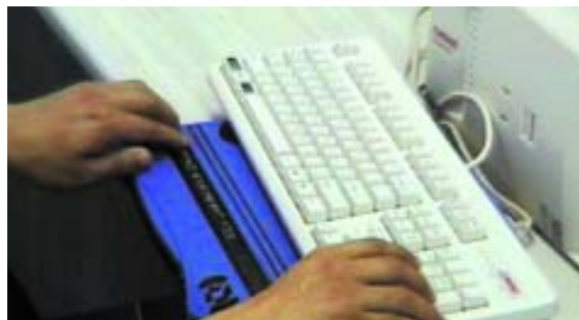
A blind student familiarizing himself with the Braille terminal (his left hand is touching the tactile screen)
