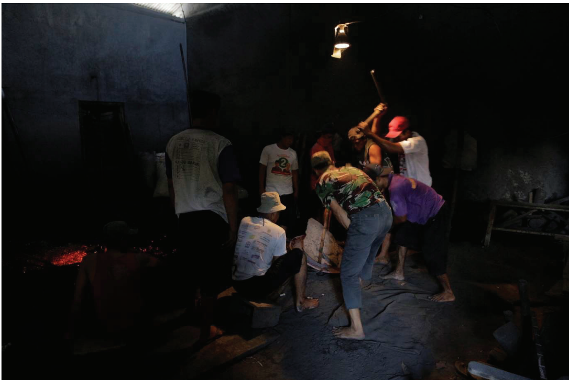
The process of making gamelan. The hammering process, three or four craftsmen in rapid rotation while another craftsman holds it steady with tongs.
