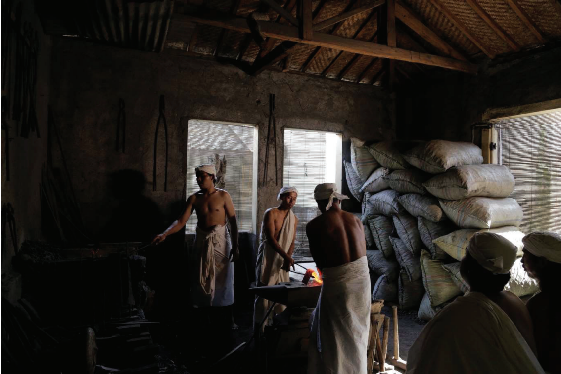
One of the Kris making steps: inserting Pamor
